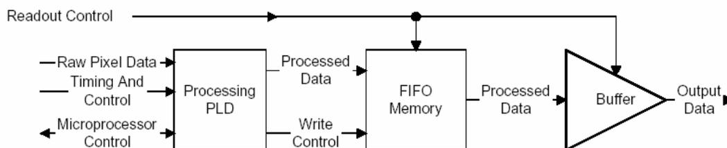
**Fig. 4.** Image Processing Architecture Block Diagram
