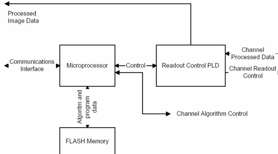
**Fig. 5.** Microprocessor/FIFO Readout Control Circuit Board Block Diagram
