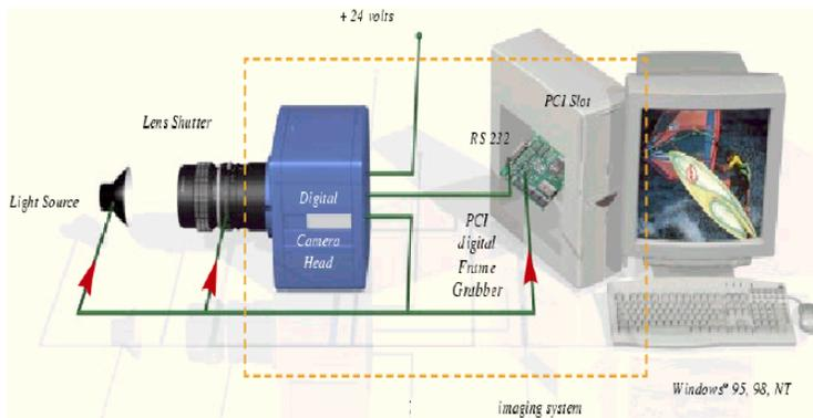
**Fig. 1.** Standard Smart Vision System (Image courtesy of Atmel Grenoble) [4]
