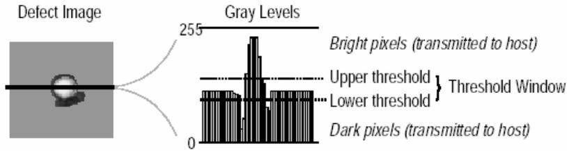
**Fig. 6.** An Example of Static Thresholding
